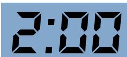
\*\* The override timer will reduce as time goes by indicating the remaining time left. When the override time expires the unit will revert to settings, prior to activating the override function. The unit will continue to take readings during the override to ensure that the unit will automatically make any required necessary ventilation adjustments at the expiry of the override.
